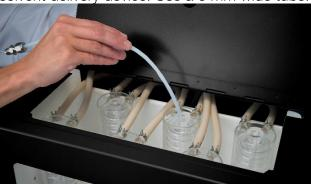
3. Place the cups with samples in the sample tray and insert that into the SoxROC Extraction Unit. Close the safety door.
