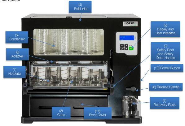
A hotplate (1) controlled by software will maintain an operator controlled temperature for the boiling and rinsing steps. This hotplate will automatically move up at the beginning of the boil and move down when reaching the drying step. The hotplate is monitored by two separate temperature systems to ensure safety.
